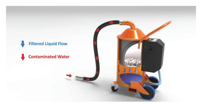
The Micro is the smallest Freddy with a 50 litre tank capacity and a 37 litre perforated steel filter basket. It comes with a 38mm or 51mm hose and a 200um filter bag as standard. With the ability to vacuum 238ltr per minute, and air flow of 3000 litre per minute, the Micro is a small but powerful addition to the range.
