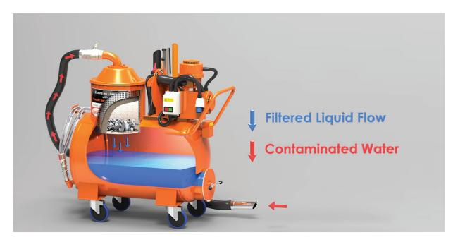
The Midi is available with either a 200 or 300 litre tank capacity, with a 37 litre perforated steel filter basket. It comes with a complete tool kit and a 200um filter bag as standard. With the ability to vacuum at 290 litres per minute and return at 130 litres per minute it offers a powerful solution to fit into narrow spaces.
