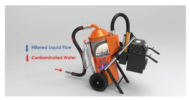
The Superminor has a 100 litre tank capacity, with a 37 litre perforated steel filter basket. With a unique tilt and lift design it offers quick and easy emptying. It comes with a complete tool kit and a 200um filter bag as standard. With the ability to vacuum at 300 litres per minute and return at 140 litres per minute it offers a powerful solution with a minimum footprint.
